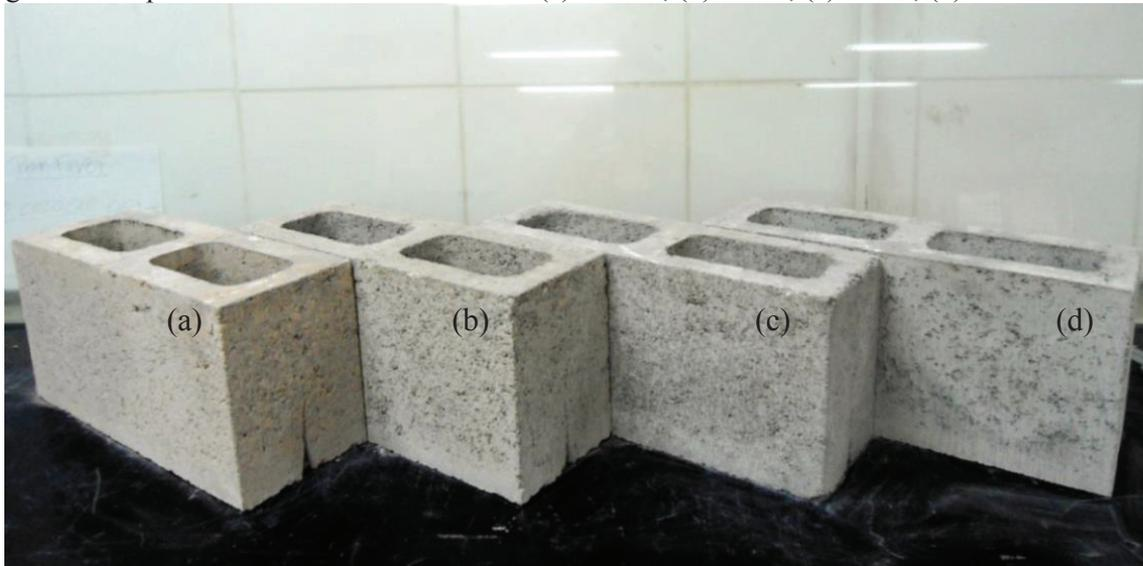
Figura 35 - Coloração dos blocos de concreto: (a) BR100; (b) BR50; (c) BR30; (d) BC.
