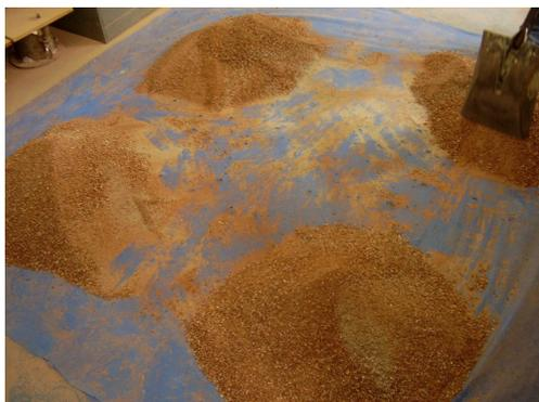
**Figura 3.20** – Quarteamento das amostras de RCD.
