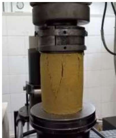
Figura 55: Ruptura de RCC100 (100x128 mm).
