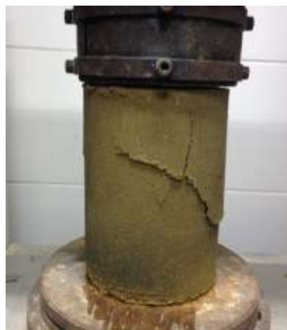
Figura 56: Ruptura de RCC91C9 (100x128 mm).
